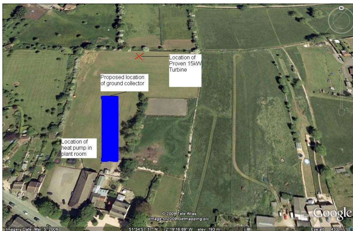
**Figure: Location of proposed wind turbine and GSHP system**
