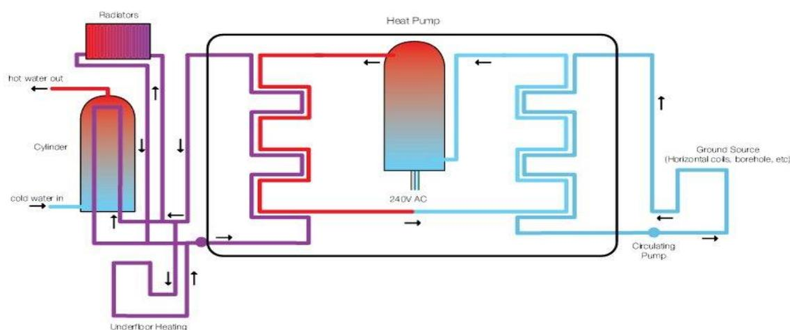
The technology in heat pumps is essentially the same whether the heat source is from the ground, the water or the air. However, as there is an inherent difference in temperature stability between these sources the overall efficiency (commonly described as the coefficient of performance – COP) will tend to vary.
