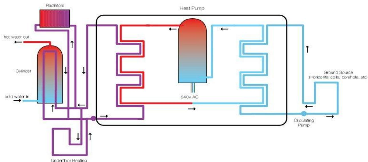
The heat pump is powered by electricity but for every one unit of electricity used, 2 - 4 units of heat energy is produced as the total amount of heat energy delivered to the building is equal to the energy input through the compressor plus the energy extracted from the heat source. As heat pumps use electricity they are not CO<sub>2</sub> neutral.
