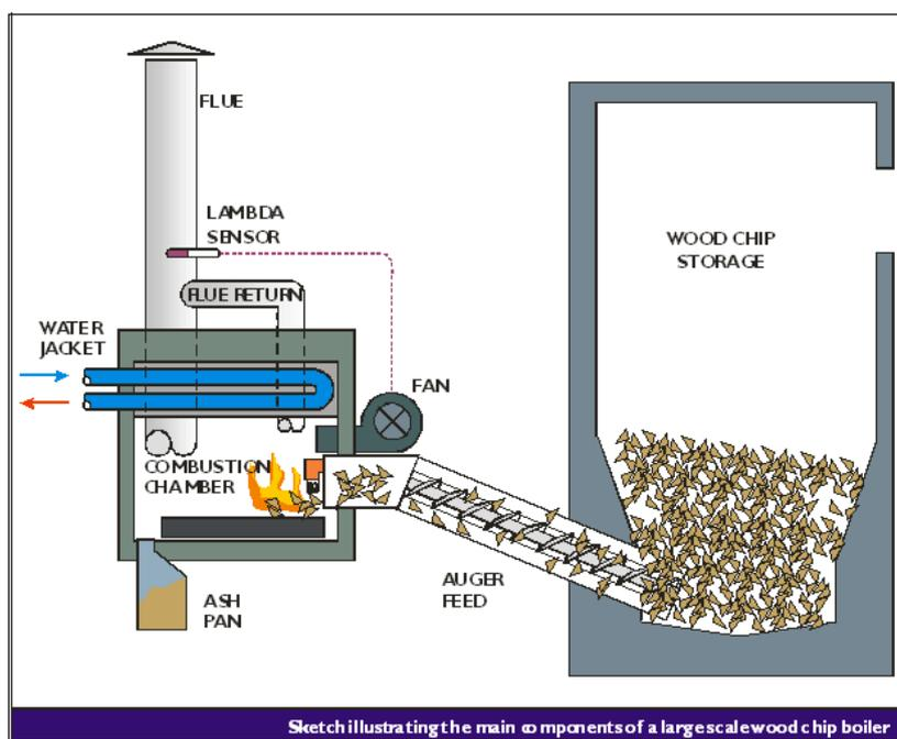
**Figure: Typical automated wood chip and store**
